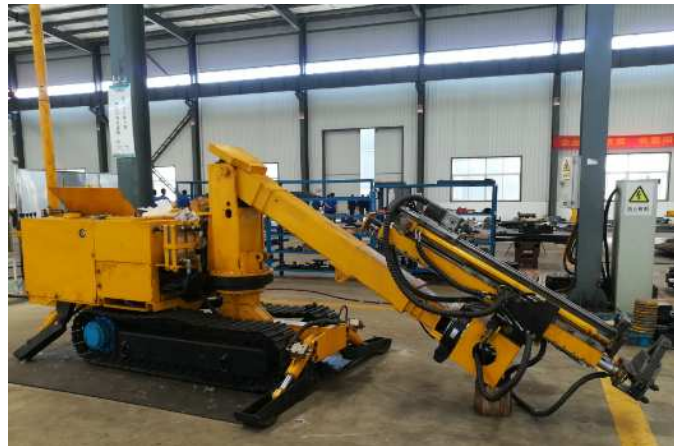
Figure 1. A hydraulic roofbolter.
