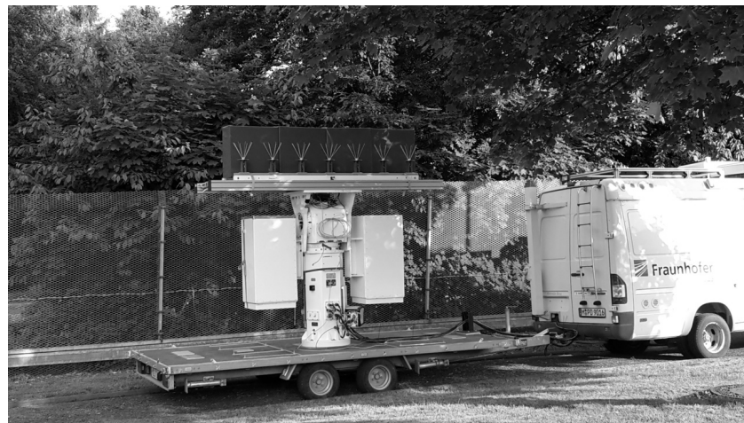
Figure 7. Picture of the bus with the trailer as the carrier platform. The uniform linear array is mounted on top of the white pedestal and steered along-track in the right-looking condition. The Radiation Absorbing Material (RAM) shielding the antennas to one side can be seen on top of the pedestal behind the antenna array.
