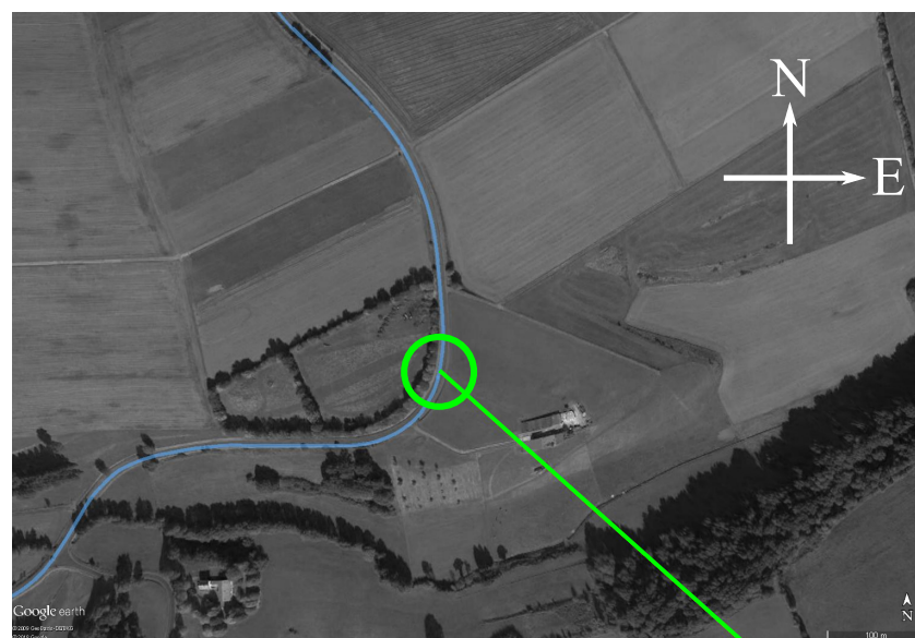
Figure 8. Picture of the trial site. The blue line indicates the trajectory of the receiver, while the green circle indicates its position at the time stamp of data evaluation. The green line indicates the baseline. Map data: ©Google, ©GeoBasis-DE/BKG 2009.
