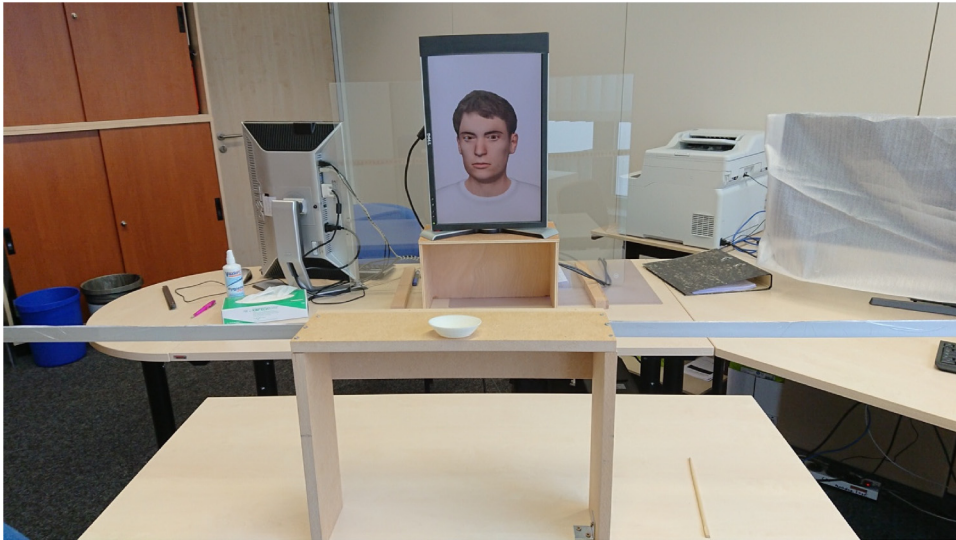
Figure 3. Setup of the experiment. Note the chin rest for the subject. The horizontal bar underneath it had cm unit values painted on the other side, only visible to the experimenter, who sat behind the display monitor, such that his/her face was occluded to the subject.
