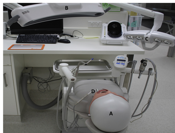
Figure 1 Showing the different components of the DentSim™. (A) Phantom Head, (B) Overhead Infrared Camera, (C) Light Source, (D) Infrared Sensor.
