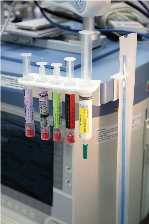
FIGURE 3: Final selective laser-sintering 3D-printed bracket and accompanying bougie holder in use. The bracket clips securely to the corner of the anesthesia machine and accepts five 10–20 mL BD syringes (standard setup including phenylephrine, ephedrine, glycopyrrolate, succinylcholine, and propofol shown).
