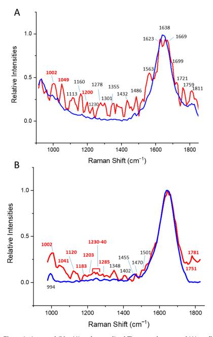
**Figure 3.** Averaged (N = 11) and normalized Time-gated spectra of (**A**) ovalbumin at 25  $^{\circ}$ C (blue) and 50  $^{\circ}$ C (red), and (**B**)  $LmTIM_{E65Q}$  at 25  $^{\circ}$ C (blue) and 86  $^{\circ}$ C (red) correspond to the individual, non-processed, and non-normalized time-gated spectra as presented in Figures S19 and S20 (i.e., raw data). Raman values of significance, as presented in Tables S6 and S7, are depicted in bold and red.
