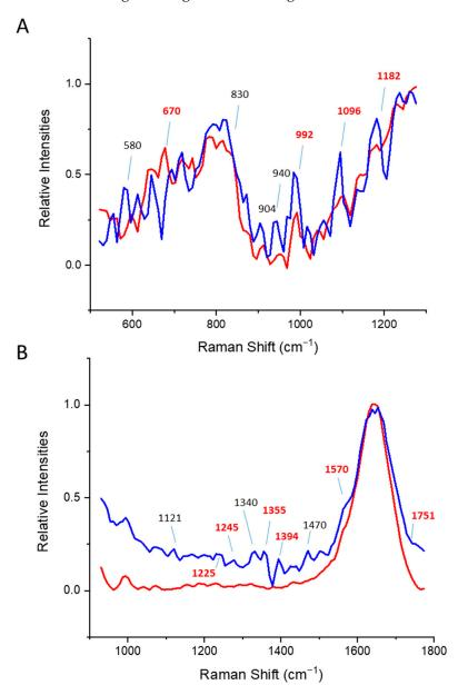
**Figure 1.** Averaged (N = 11) and normalized time-gated spectra of pepsin at 25  $^{\circ}$ C (blue) and 65  $^{\circ}$ C (red). (**A**,**B**) correspond to the individual, non-processed, and non-normalized Time-gated spectra as presented in the left and right panes in Figure S10. (i.e., raw data). Raman values of significance, as presented in Table S4 (supplementary data), are depicted in bold and red.
