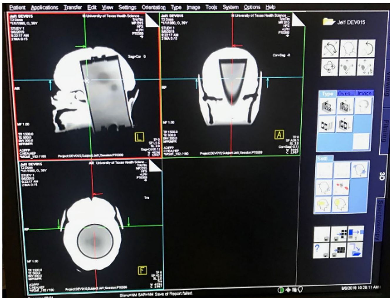
FIGURE 7 The irradiated Prime phantom scanned on 1.5 T MR unit. The top left image allows you to see how the cylindrical gel insert was placed into the hollow phantom. The remaining space around the gel is water
