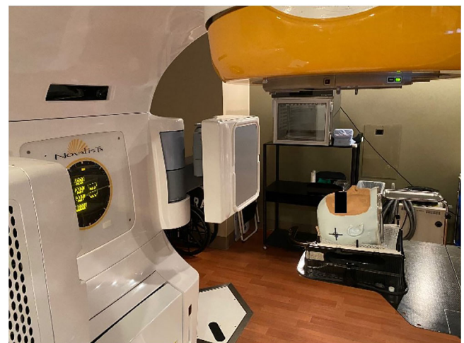
FIGURE 4 Prime phantom setup below the Varian Novalis TX (Varian Medical Systems, Palo Alto, CA) for end-to-end testing
