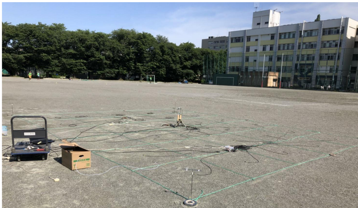
Figure 1. Experimental setup for obtaining training and validation data. MOX gas sensors are placed in each cell marked by the green strings. The anemometer can be visibly seen in the center.
