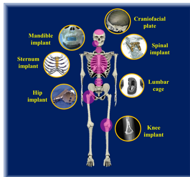
Figure 7. Craniofacial plate implant Ti-6Al-4V DMLS [161], mandibular implants [162], spinal [163] and sternum [164] implants, lumbar cage [165], hip [166], and knee implants [167]. Reprinted under copyright CCBY-NC-ND 4.0 license.
