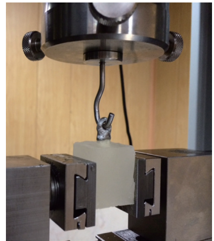
Fig. 5. Load application parallel to the longitudinal axis of the tooth at a crosshead speed of 0.5 mm/min.
