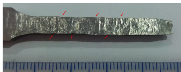
Figure 15. Surface of the calibrated longitude of the tensile specimen after being tested. Red arrows show the striations.
