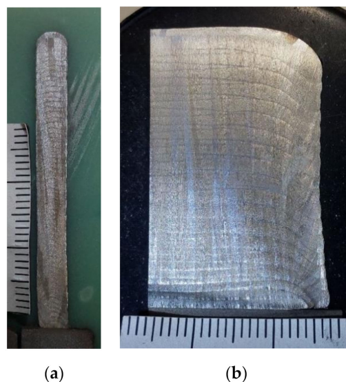
Figure 4. Cross-section of the additive material perpendicular (a) and parallel to the layers (b).
