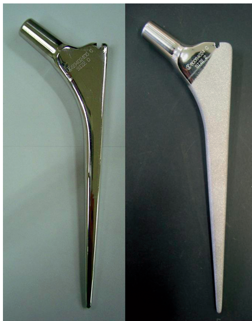
Figure 1. Collarless double-taper (CPT) stems. A polished stem is shown to the left and a matt-processed rough stem is shown to the right.
