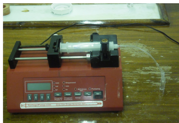
Figure 5. Semi automated device for obtaining breakthrough parameters.
