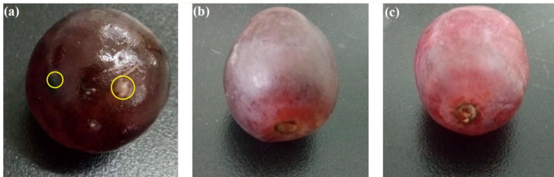
Figure 14. Preservation of red grape packed in different materials at 37 °C for 6 days: (a) plastic wrap; (b) pure chitosan film; (c) chitosan-TiO 2 film. Reprinted from [133] with permission from Elsevier.
