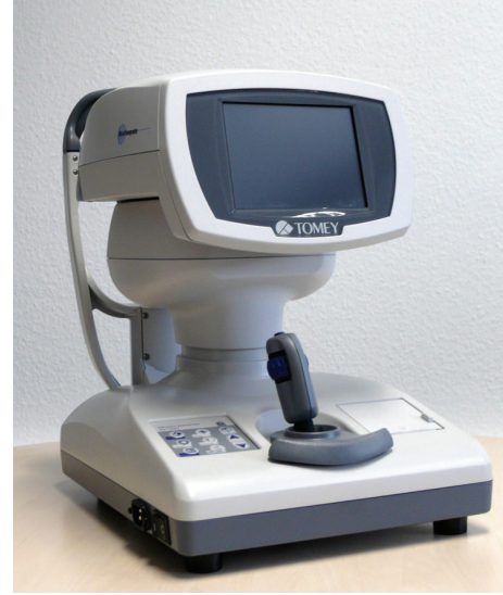
FIGURE 1: The OA-1000 by Tomey is a new optical biometer designed to measure axial length, anterior chamber depth, and corneal thickness.
