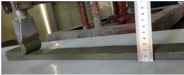
Figure 1. View of additive construction by extrusion test.
