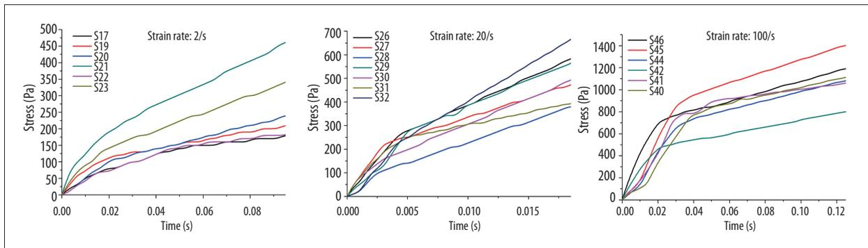
**Figure 2.** The history curve of Lagrange stress for the infant porcine brainstem specimen at the dynamic tensile tests. A total of 6 tests were conducted successfully at the stretch speed of 10 mm/s (strain rate 2/s), 7 at the stretch speed of 100 mm/s (strain rate 20/s), and 6 at the stretch speed of 500 mm/s (strain rate 100/s).
