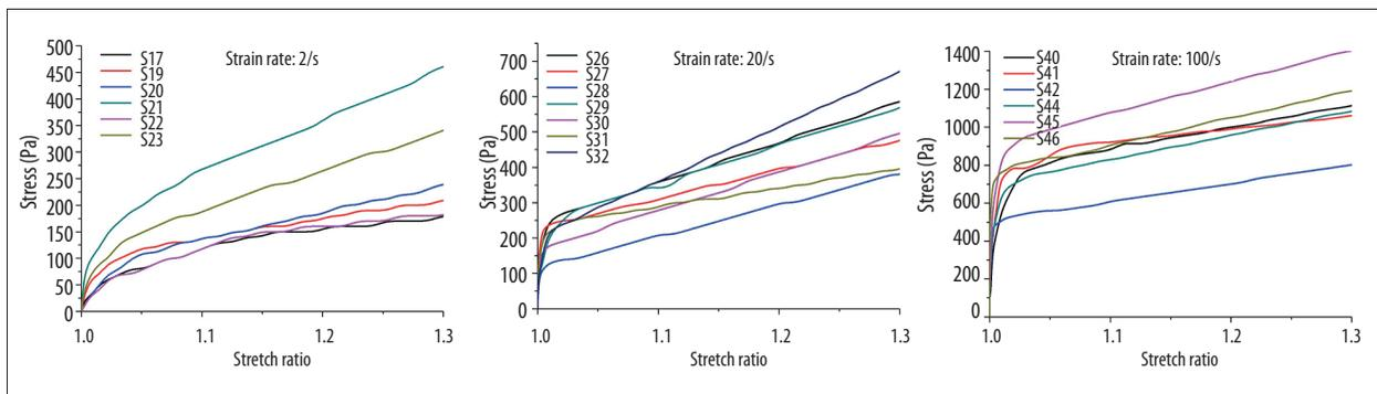
**Figure 3.** The curve of Lagrange stress-versus-stretch ratio for the infant porcine brainstem specimen at the dynamic tensile tests. A total of 6 tests were conducted successfully at the stretch speed of 10 mm/s (strain rate 2/s), 7 at the stretch speed of 100 mm/s (strain rate 20/s), and 6 at the stretch speed of 500 mm/s (strain rate 100/s).
