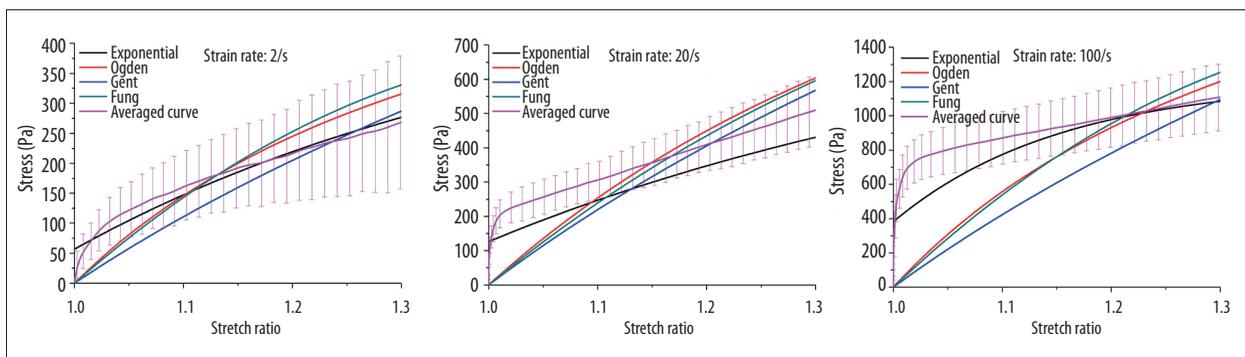
**Figure 4.** The curve fitting of Fung, Ogden, and Gent strain energy function, and exponential model for the average experimentally acquired data of stress-versus-stretch ratio at each test group. The adjusted R-Square of the model fitting the experimental data up to the strain of 30% at the dynamic strain rate is  $0.820 \leq R^2 \leq 0.933$  in Fung,  $0.774 \leq R^2 \leq 0.940$  in Ogden,  $0.650 \leq R^2 \leq 0.922$  in Gent, and  $0.852 \leq R^2 \leq 0.981$  in exponential model.
