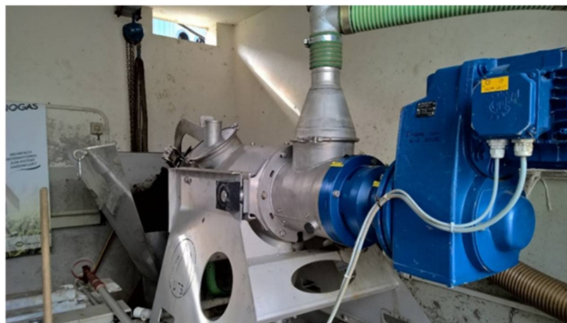
Figure 1. A filter screw press used for the digestate separation at the full-scale research biogas plant of University Hohenheim “Unterer Lindenhof”.
