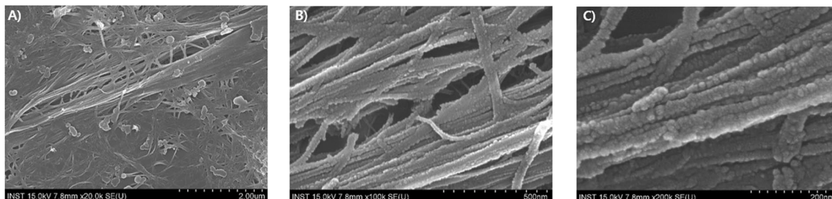
Figure 3. SEM images of silicified phage. LAR5 phage at (A) low (20k), (B) medium (100k), and (C) high (200k) magnification after silicification.
