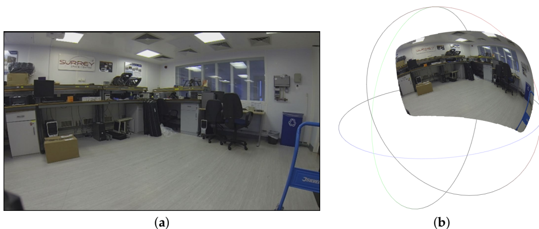
Figure 7. Image of an indoor laboratory environment illustrated as a flat array (a); and projected onto a unit sphere using its intrinsic lens model (b).
