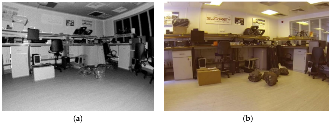
Figure 10. Image produced from LIDAR intensity measurements (a) of the laboratory setup (b).
