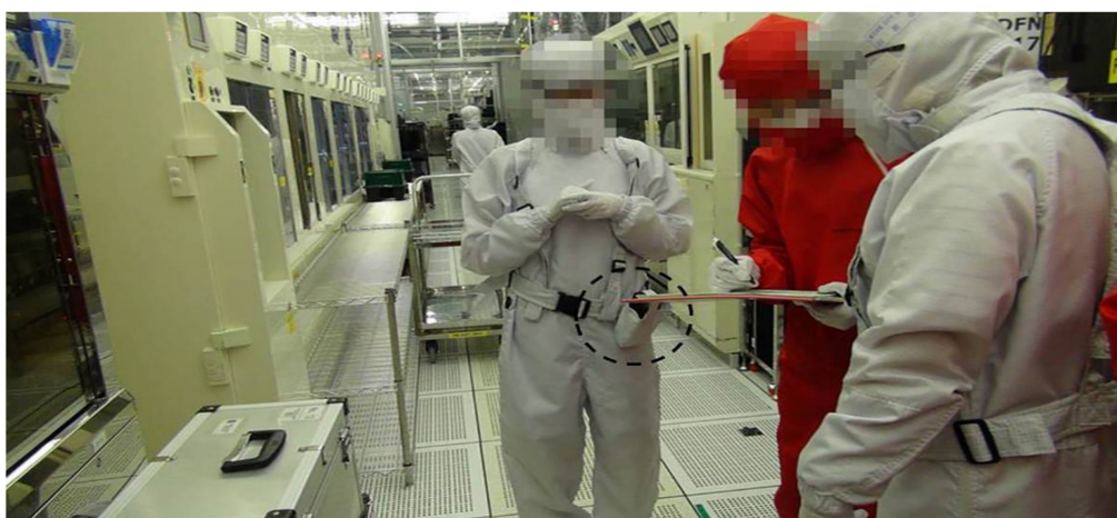
Figure 1. Semiconductor worker wearing portable ELF-MF meter on the waist, indicated with dashed black circle.
