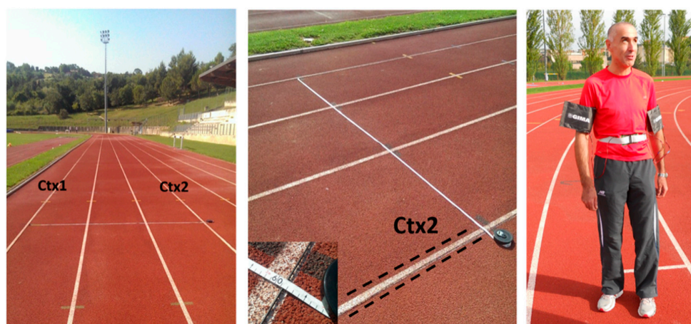
Figure 6. The blind athlete equipped with the electromagnetic sensor at an outdoor running track. Ctx1 and Ctx2 indicate the two wires generating the magnetic field.
