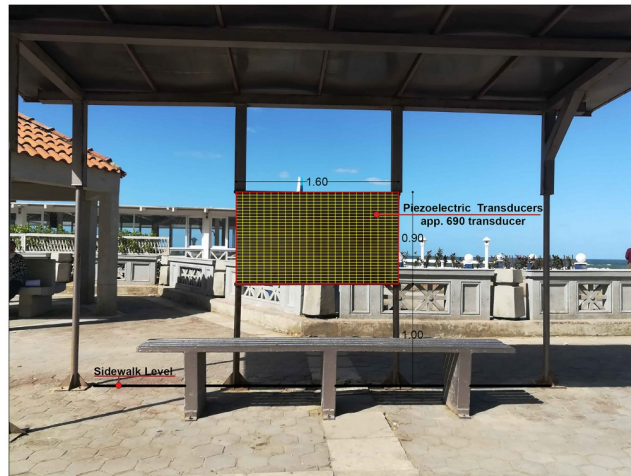
Fig 13. The proposed area to place the piezoelectric transducers at the bus stop of Cleopatra Station as an example. The area is about 1.45 m 2 and it takes about 690 QB220-503YB transducers to cover this selected area (Researcher, 2018).
