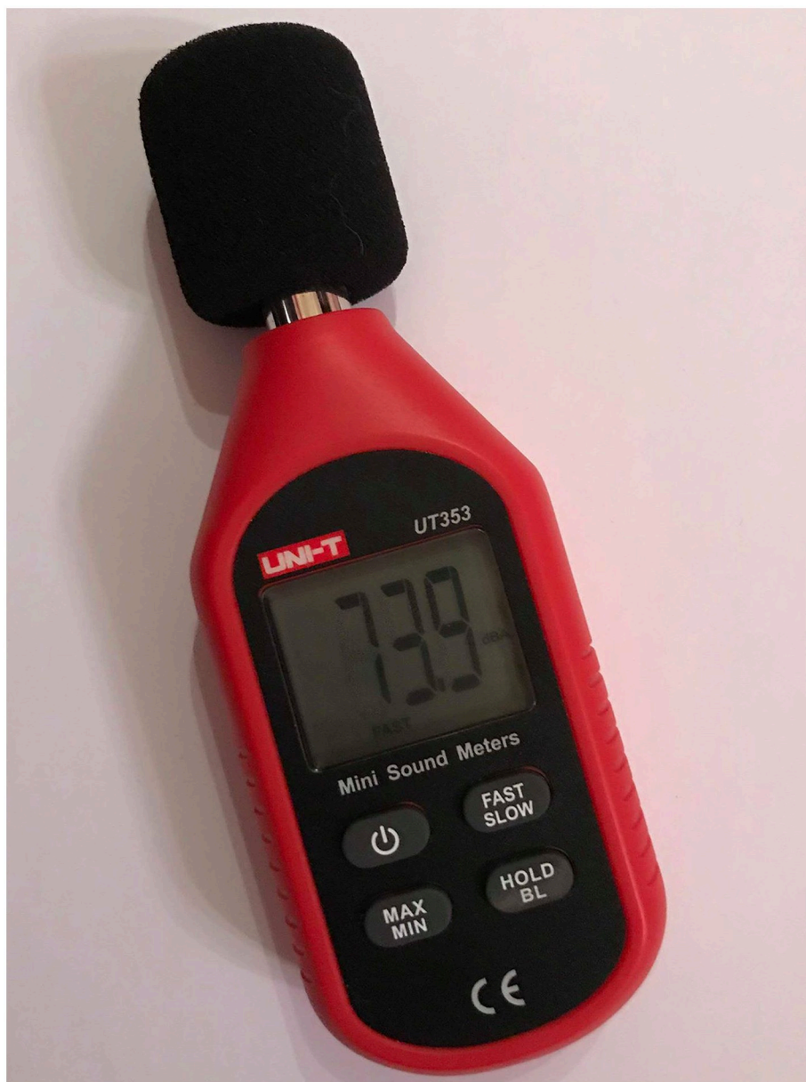
Fig 6. The UT 353 digital sound meter device. (Researcher, 2018).
