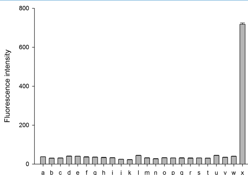
Figure 5. Fluorescence dependence of probe 1 ( 7.5 \mu\text{M} ) on HClO ( 30 \mu\text{M} ) and other different substances ( 500 \mu\text{M} except for specifically being labeled): (a) only probe, (b) \text{K}^+ , (c) \text{Na}^+ , (d) \text{Ca}^{2+} , (e) \text{Mg}^{2+} , (f) \text{Al}^{3+} , (g) \text{Zn}^{2+} , (h) \text{H}_2\text{O}_2 , (i) TBHP, (j) \cdot\text{OH} , (k) \cdot\text{O}^t\text{Bu} , (l) ^1\text{O}_2 , (m) ascorbic acid, (n) \text{O}_2^{\cdot-} , (o) \text{NO}_3^- , (p) \text{NO}_2^- , (q) Cys, (r) Hcy, (s) GSH, (t) \text{ONOO}^- , (u) \text{Fe}^{2+} , (v) \text{Fe}^{3+} , (w) \text{Cu}^{2+} ( 100 \mu\text{M} ), and (x) HClO.
