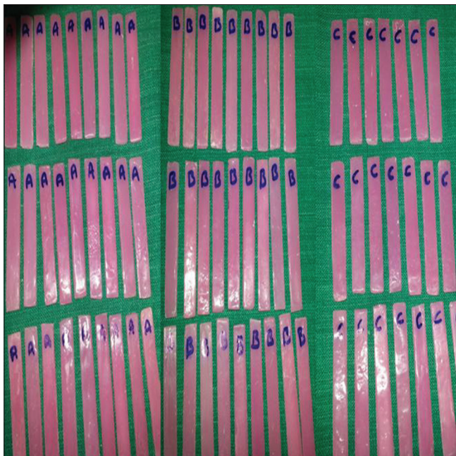
Figure 4: Finished and polished specimens
