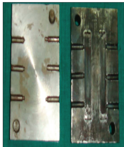
Figure 1: Metal mold to make test samples
