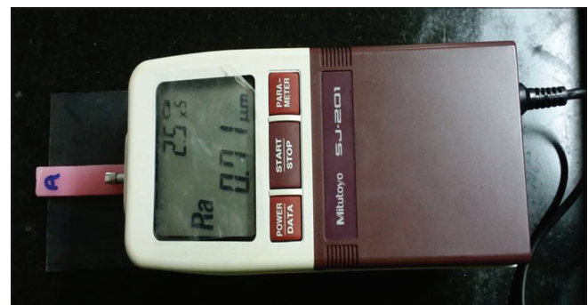
Figure 7: Testing of surface roughness of specimen
