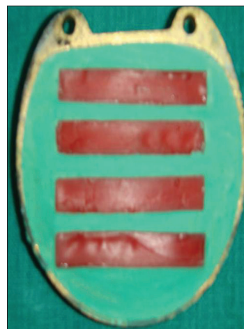
Figure 2: Invested wax blocks in dental stone
