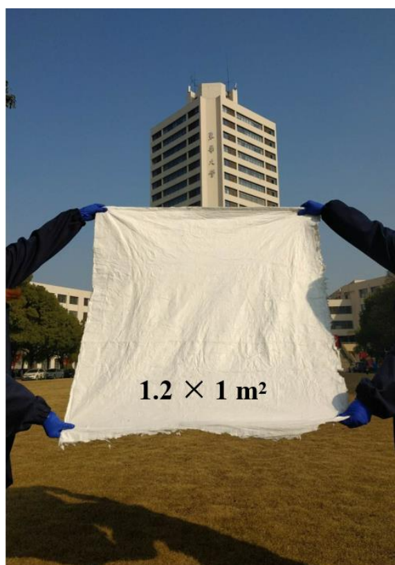
Figure S6. A large-scale ceramic NF membrane with an area of 12000 cm 2 , related to Figure 2(a).
