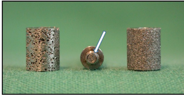
Fig. 3. Exemplary porous (left) and solid, sand-blasted (right) Ti-6Al-4 V implants with a height of 7.0 mm and a diameter of 5.6 mm. The push-out device (middle) is 1.0 mm undersized in diameter compared to the implants to avoid contact with the bone during the push-out process. A central mandrel (arrow) of the device fits snugly into the central drill chanal of the implants.
