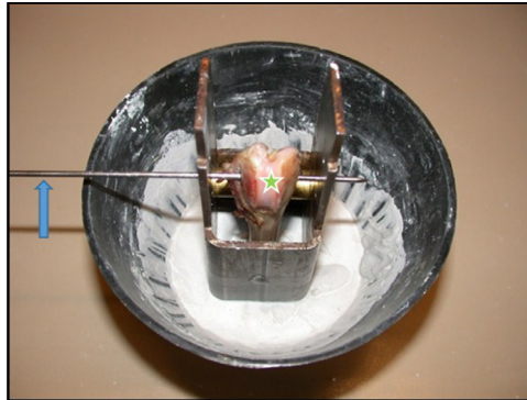
Fig. 5. Positioning of the specimen (star) in the sawing jig. The distal femur was aligned using the central spike wire (arrow) in order to ensure a perpendicular cutting plane to the longitudinal axis of the implant. Finally, the distal femur was covered with gypsum for the further cutting process.
