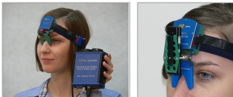
Figure 2. The head-mounted JAZZ-novo eye tracker [30] as used in the research.
