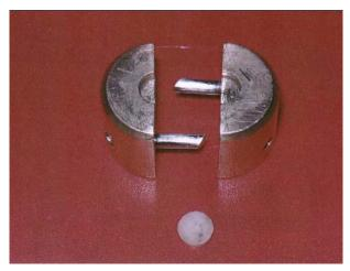
Fig 1. The metallic mold used for preparing the specimens.
