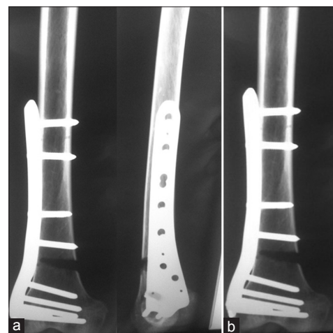
Figure 4: (a) Pre test X ray showing distal femur specimen with metaphyseal osteotomy implanted with distal femoral locking plate. (b) Post test X ray showing distal femoral locking plate specimen – Remained stable after 50,000 cycles
