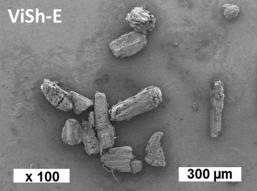
Figure 1. Scanning electron microscopy (SEM) pictures of vine shoots fillers.
