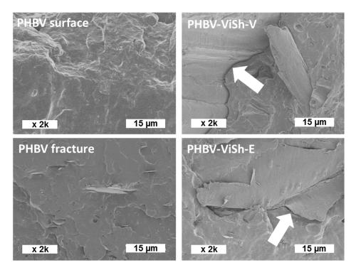
**Figure 4.** SEM pictures of the poly(3-hydroxybutyrate-3-hydroxyvalerate) (PHBV) surface and fracture (on the left) and SEM pictures of the PHBV-based composite fractures (filler content of 20 wt %) (on the right). White arrows show the matrix/filler interface.
