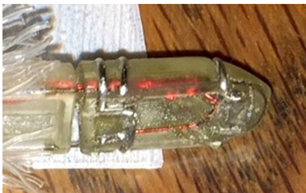
Figure 3 The walker wrapped with silver electrodes forming a dipole pair that allows it to be guided by SEMDM.
