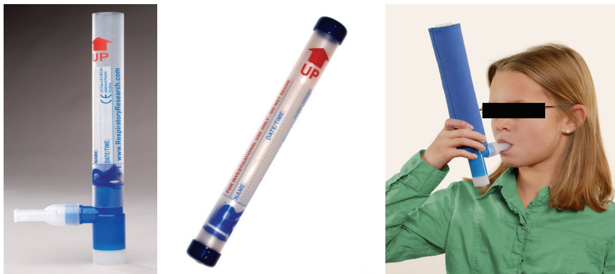
FIGURE 3: RTube device for exhaled breath condensate (EBC) collection (Respiratory Research, Inc., USA). RTube disposable collection system consists of a large Tee section (from polypropylene (PP)), which separates saliva from the exhaled breath, an one-way valve (from silicone rubber), and a PP collection tube, which is cooled by a cooling-sleeve placed around. RTube is portable and can be used by unsupervised subjects at home ( published with permission from Respiratory Research, Inc., USA ).
