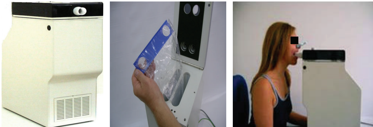
FIGURE 1: EcoScreen 2 device for exhaled breath condensate (EBC) collection (FILT Lungen-& Thorax Diagnostik GmbH). EcoScreen 2 electrically refrigerates exhaled air, conducted through a lamellar PTFE coated aluminum double lumen system. EBC is formatted in a disposable polyethylene bag (at approximately -10^{\circ}\text{C} ). It also allows the fractionated collection of EBC from different areas of the bronchial tree into two disposable polyethylene bags, so that the dead space condensate which contains biomarkers of no clinical relevance can be discarded. The device is not portable and weighs 20 kg (published with permission from FILT Lungen-& Thorax Diagnostik GmbH).
