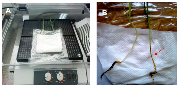
Fig. 1. A Photographs of a sandwich filter paper method; (A) Incubation of barley seedlings (cv. WI 2291) after C. sativus inoculation. (B) Infected seedling with brown lesions (arrow) after 5 days of inoculation (right side), and the clean control (left side).
