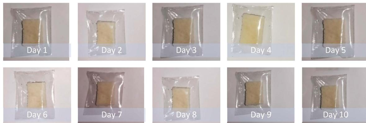
**Figure 8.** The bread piece was packaged in PVA with 15 % GF films. This sample was placed in an open atmosphere (30 °C and 50% RH) for 10 days to see the effect of the packaging.
