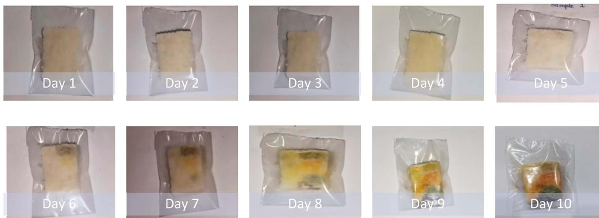
**Figure 7.** The bread piece was packaged in commercial polyethylene films and placed in an open atmosphere in ambient conditions (30 °C and 50% RH) for 10 days to see the effect of the packaging on the degradation of the bread piece.
