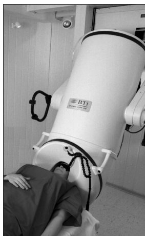
Figure 2: Patient in MEG machine. The cylinder contains the liquid helium. The SQUID sensors in the machine are located in close proximity to the patient's head
