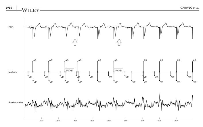
**FIGURE 5** Example behavior during PACs. A late coupled PAC (left arrow) is tracked without loss of AV synchrony while an early coupled PAC (right arrow) is not tracked since it is in the blanking period (PVAB). AV, atrio-ventricular; PAC, premature atrial contraction; PVC, premature ventricular contraction
