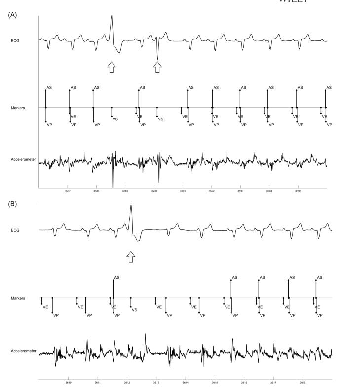
**FIGURE 4** Example behavior during PVCs. (A) shows minimal disruption in atrial sensing after a PVCs (arrow). (B) shows multiple beats are needed to re-establish AV synchrony since sinus beat occurred after ventricular pace beats. AS, atrial sense; PVC, premature ventricular contraction; VE, end of A3 (ventricular) window; VP, ventricular pace
