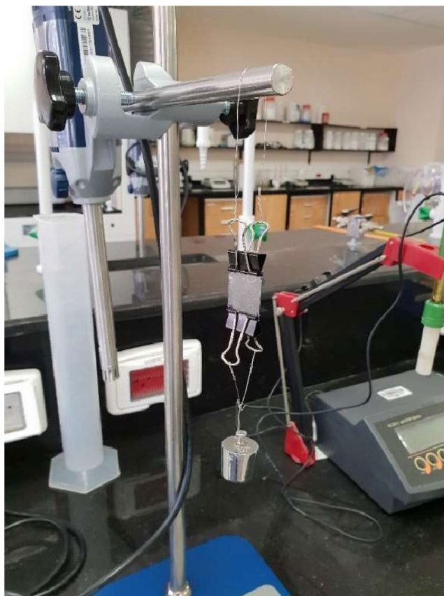
Figure 14. Young's modulus test performed manually.
