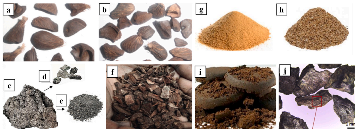
Fig. 3. Morphology of lignocellulosic LWA: a. Uncrushed OPS; b. Crushed OPS [76]; c. POC fragment taken from the factory, d. POC coarse aggregate, e. POC fine aggregate [77]; f. coconut shell [78]; g. fine sawdust; h. coarse sawdust [79]; i. spent coffee ground [80]; j. expanded cork granules [23].
