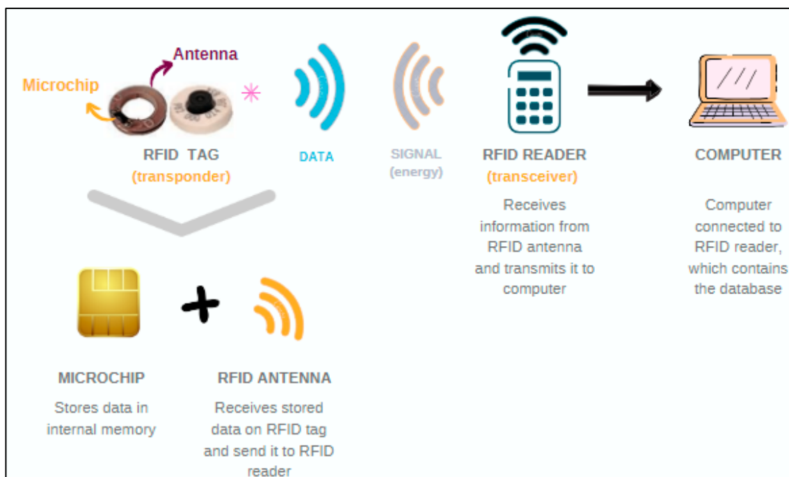
Figure 2. Basic electronic identification (EID) using radiofrequency identification system (RFID) transmission. Note that the RFID tag can have different presentations. This figure shows an example of an electronic ear tag. * Could also be a collar or a pedometer as a transponder. Own source.
