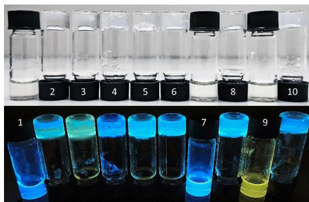
Figure 4. Water/organic solvent mixtures of 1 (10 mg/mL) under ambient light (top) and under 365 nm UV-light irradiation (bottom), 24 h after heating to 80 ^\circ\text{C} . Co-solvents: 1) MeOH; 2) EtOH; 3) i -PrOH; 4) HFIP; 5) acetone; 6) acetonitrile; 7) DMSO; 8) DMF; 9) THF; 10) 1,4-dioxane.
