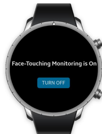
Figure 1. The smartwatch app user interface. The app collects continuous raw accelerometer data as long as it is on. The “TURN OFF” button allows the user to stop collecting data. The text above the button confirms that the data are being collected.
