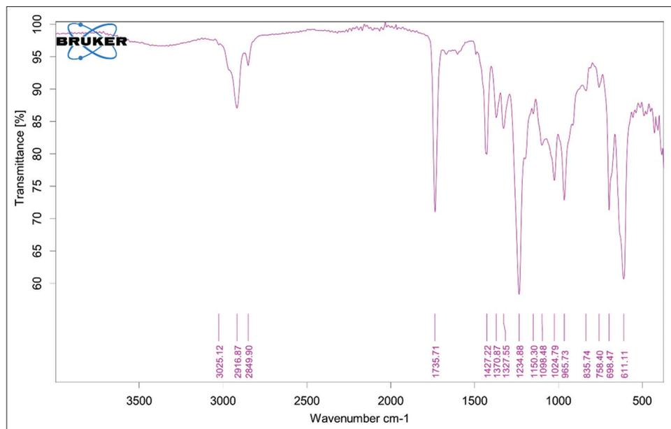
Figure 4: FTIR spectra of Endure square (ES)
