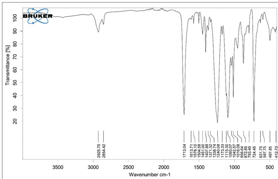
Figure 2: FTIR spectra of Centri Form-Clear rigid material CFCRM
