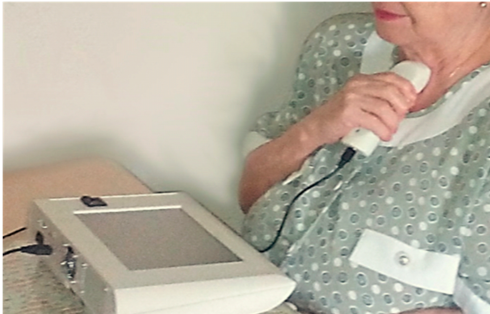
Figure 2. Photograph of a subject using the respiratory sensor at home during the process of respiratory sounds acquisition at the suprasternal notch. The base-station assistant steps the user through the process. The process is guided by the base station using visual and voice instructions for guidance.
