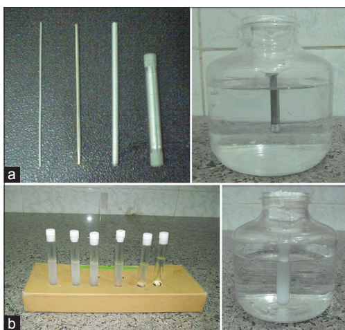
Figure 3: (a) The samples which scanned in order to determine the system spatial resolution. (b) The samples which scanned in order to investigate the system contrast resolution
