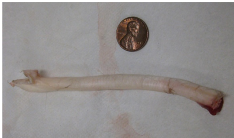
Figure 12 Hind leg deer tendon, removed for testing.
