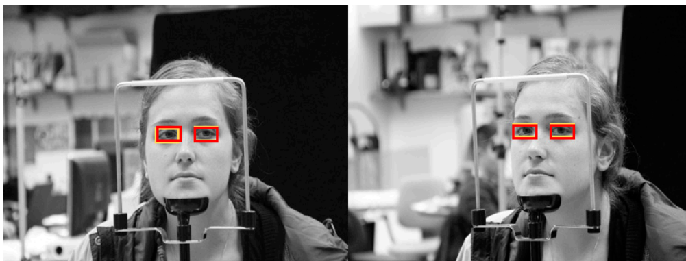
Figure 25. Example of correctly detected eyes by proposed method (Yellow and red rectangles show the ground-truth and detected boxes, respectively).
