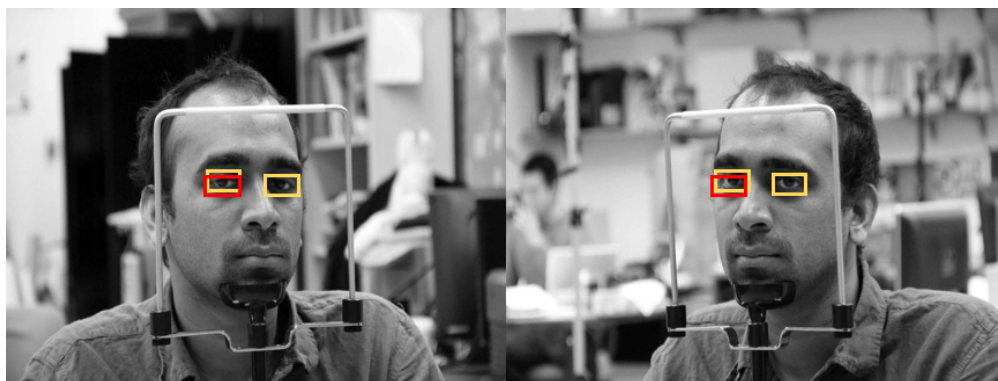
Figure 26. Example of incorrectly detected eye by proposed method (Yellow and red rectangles show the ground-truth and detected boxes, respectively).
