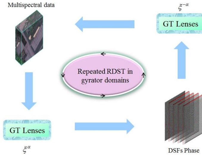
Figure 2. The schematic diagram of random devil's spiral Fresnel transform.
