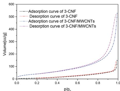
Fig. 6 N<sub>2</sub> adsorption–desorption isotherms of 3-CNF and 3-CNF/MWCNTs.
