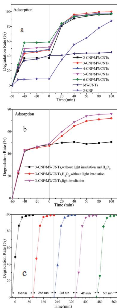
Fig. 8 (a) Degradation rate of MB in the presence of the different samples with H<sub>2</sub>O<sub>2</sub>, (b) removal rate of MB in the presence of 3-CNF/MWCNTs without light irradiation, 3-CNF/MWCNTs + H<sub>2</sub>O<sub>2</sub> without light irradiation and 3-CNF/MWCNTs with light irradiation and (c) repetitive use of 3-CNF/MWCNTs.
