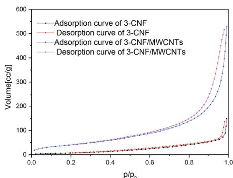
Fig. 6 N<sub>2</sub> adsorption-desorption isotherms of 3-CNF and 3-CNF/MWCNTs.
