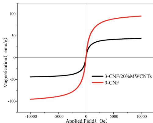
Fig. 7 Magnetic hysteresis loops for 3-CNF and 3-CNF/MWCNTs.
