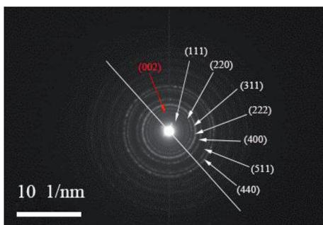
Fig. 2 Selected area electron diffraction pattern of 3-CNF/MWCNTs.
