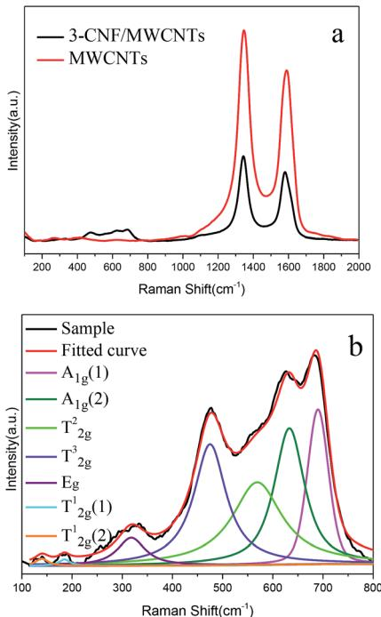
**Fig. 4** Raman spectra (a) MWCNTs and 3-CNF/MWCNTs and (b) 3-CNF/MWCNTs in the low wavenumber range of 100–800 cm<sup>-1</sup>.
