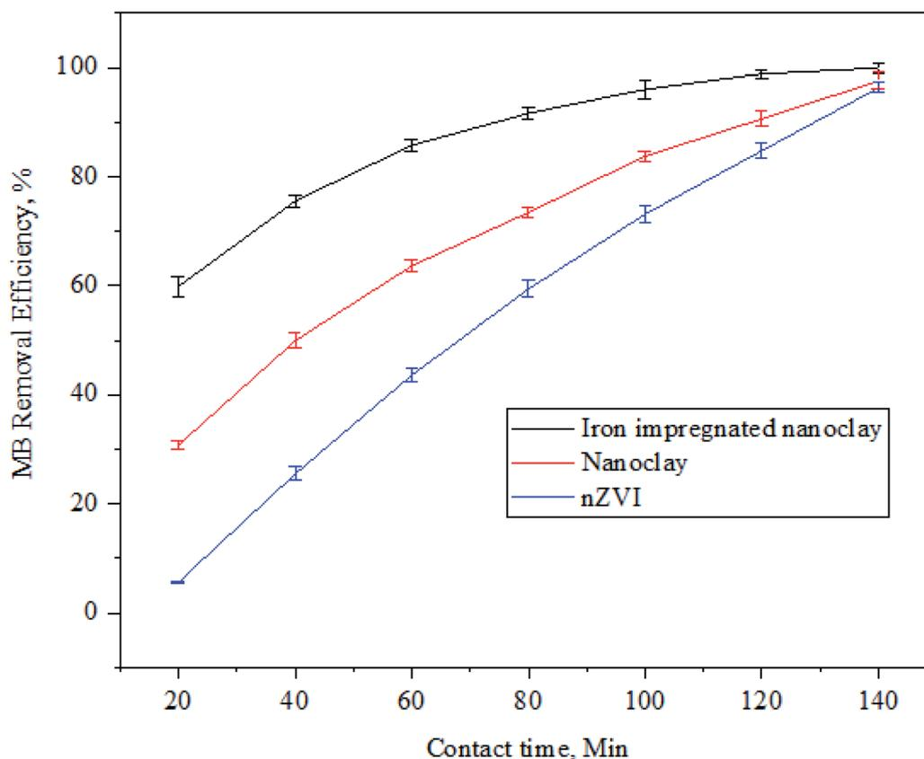
Fig. 18 Trends in methylene blue dye adsorption with contact time ( $n = 3$ , adsorbent dose:  $60 \text{ mg}$ , MB concentration:  $60 \text{ ppm}$ , temperature:  $30 \text{ }^\circ\text{C}$  and pH: 7.5).
