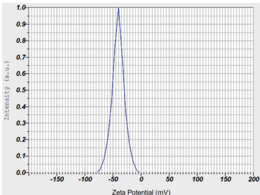
Fig. 15 Zeta potential of iron impregnated nanoclay.
