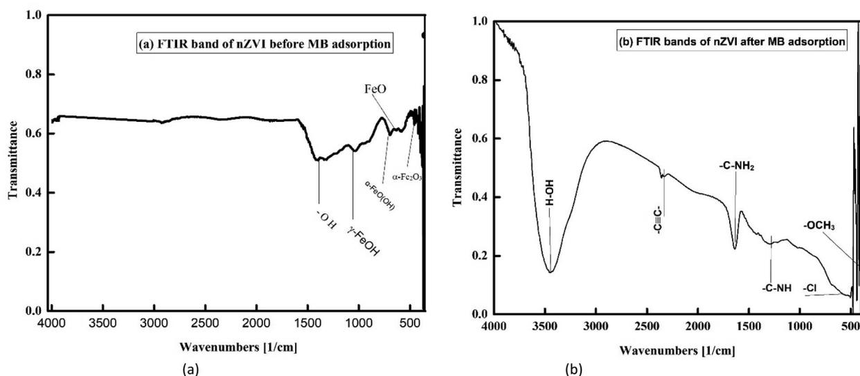
Fig. 7 FTIR Images of nZVI: (a) before MB adsorption, (b) after MB adsorption.
