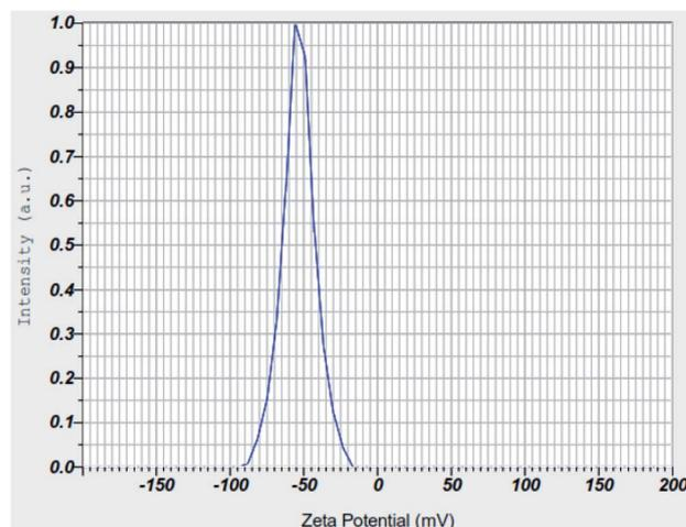
Fig. 14 Zeta potential of nanoclay.
